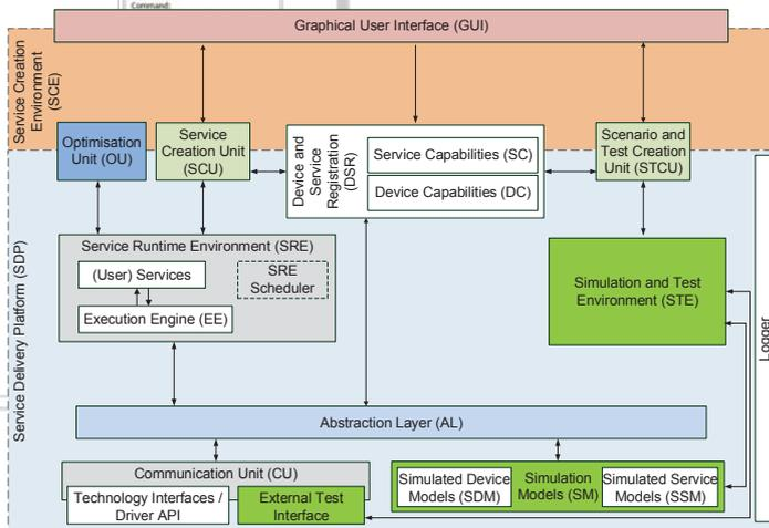
An Abstraction Layer integrated into the SMF allows the connection of different Smart Home systems to the platform.
