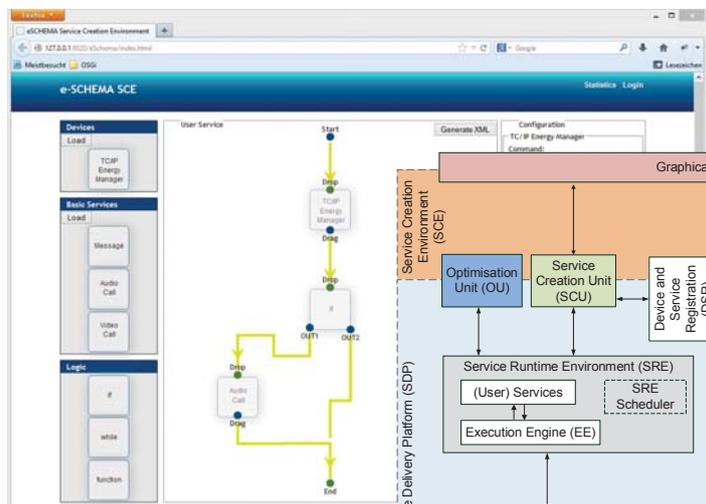
Through a SCE (Service Creation Environment), the user is able to design value added services for controlling of his Smart Home by graphically combining of device blocks delivered by the manufacturer of home appliances. These services are transformed into a formal notation and interpreted/ executed by the Service Delivery Platform (SDP).
