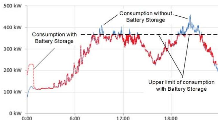
An exemplary simulated scenario covers "avoidance of peak load" by using battery storages for a community of 1000 households. The results shown on the left side indicate that, for a 20% peak load reduction (from 45.9kW to 36.7kW), already 23 standard battery storages are sufficient, that means only 2.3% of households would have to be equipped with one battery storage.
