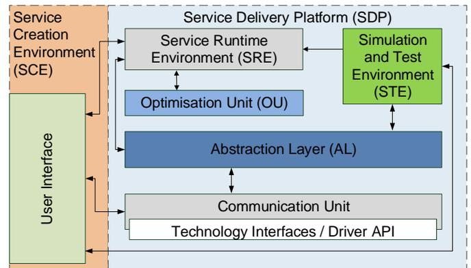
Fig. 2. Overview of relevant parts of SMF
