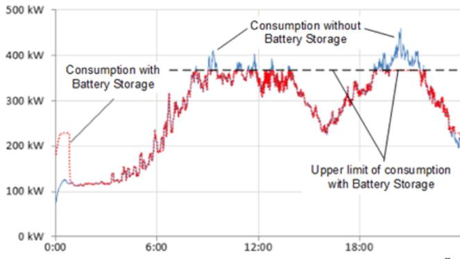
Fig. 7. Results peak load reduction using Battery Storages
