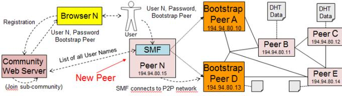
Fig. 3. Joining the P2P networked Energy-Community
