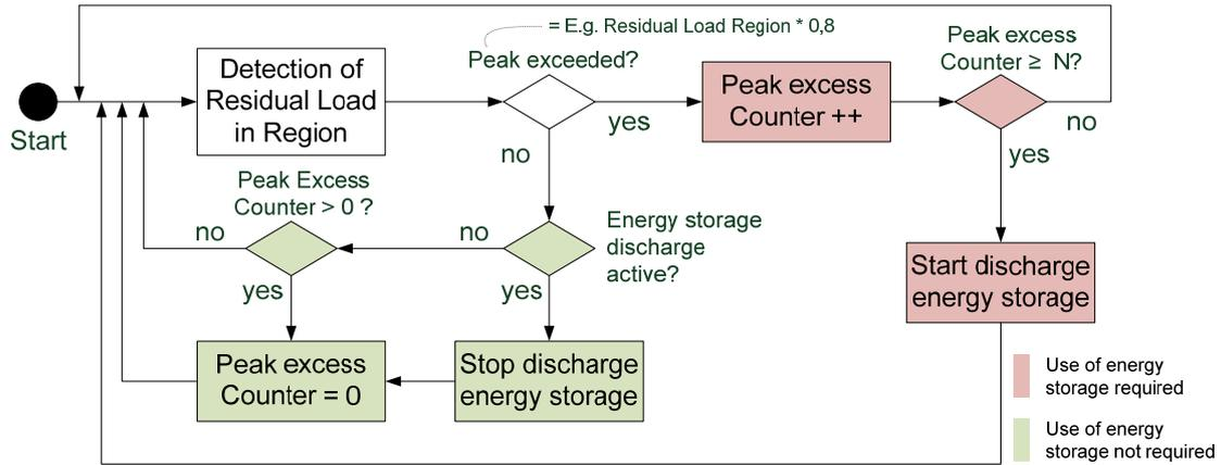
Figure 3. Section of algorithm for peak load reduction
