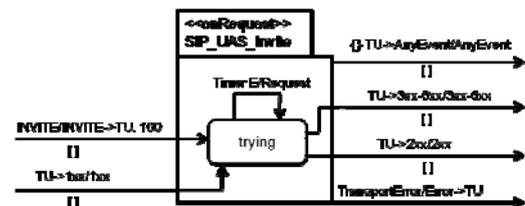
Figure 4. Structure of the finite state machine SIP\_UAS\_Invite
